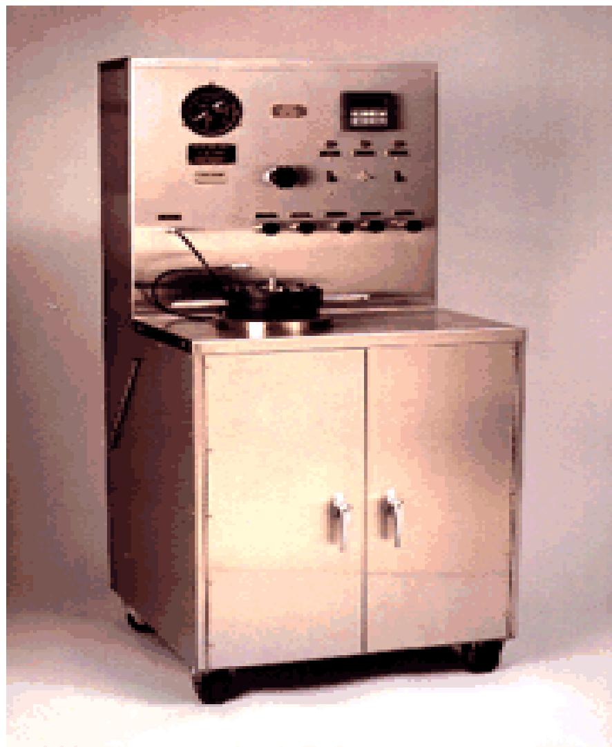
IMAGE ٧: HIGH TEMPERATURE-HIGH PRESSURE CURING CHAMBER
